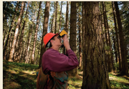
Collecting accurate tree heights with a laser rangefinder. Photo by Bob Crum
