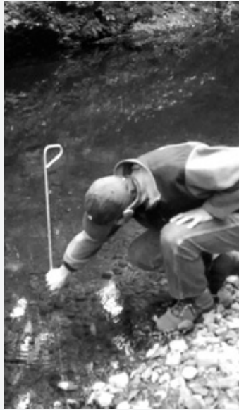
Guild member Linwood Gill testing depth to armor layer in Flynn Creek, CA.
